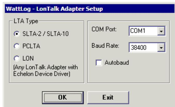
Then choose the **SLTA-2 / SLTA-10** from the dialog box below and select the correct COM port and baud rate (38400). If you are using a COM port number that doesn't appear in the drop-down, you may type your own COM port number.
