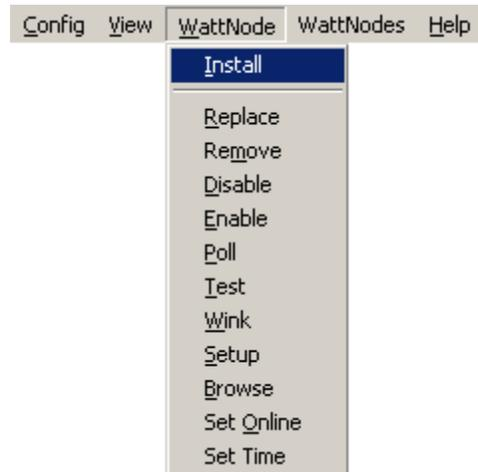
This allows you to install, maintain and trouble shoot configure WattNodes on your network. The selected command is applied to whichever WattNode is highlighted in the grid.
