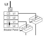
3) To open the CT, squeeze the knurled panels, then pull and rotate the top open.
